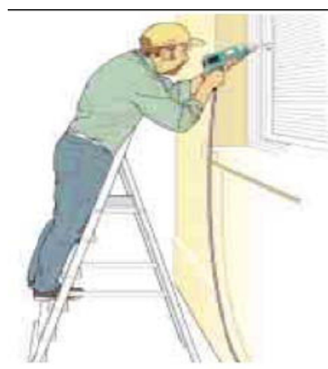
Correct – steps facing work activity
