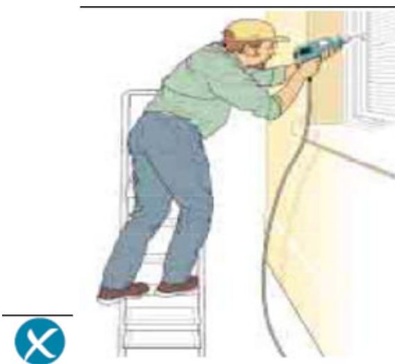
Incorrect – steps side on to work activity
